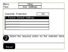
2 Press **RECALL** to recall the instrument default settings. The instrument display will blank for a few seconds while the settings are recalled and the status display will indicate stored settings number 0 recalled.
